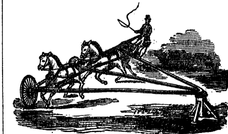
PATENT AMERICAN HORSE-BREAK. The engraving shows the construction, which is very simple, and it seems to us as well calculated to accomplish the work designed, as the horse can do no injury to himself or the driver,—can neither rear
