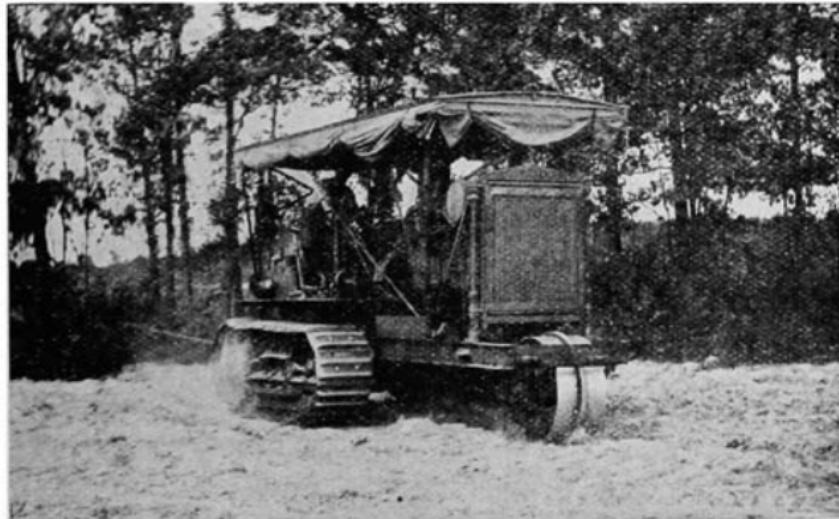
The Holt Caterpillar Tractor. Removes the stump as well as the tree.
