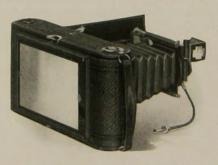
When substituted for the usual autographic backs on No. 3A Autographic Kodaks, Regular and Special, Combination Backs adapt these cameras to double plate holders. The photographer then has the advantage of ground glass focusing and, if he so desires, can make one or two exposures and develop them at once.
