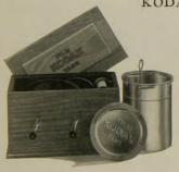
These outfits afford the easiest, most reliable means of developing film negatives. No darkroom is necessary. By means of the light-tight box the film is transferred to a reel, being covered at the same time by a protecting apron. Reel, film and apron are immersed in the solution cup and development is made according to directions which accompany each outfit.
