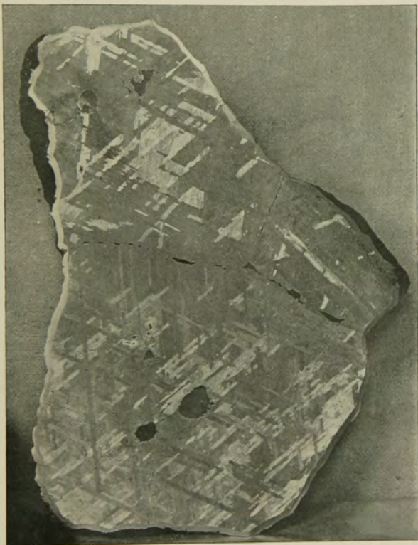
Section showing Widmanstätten figures. One-third actual size.
