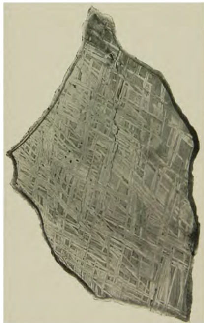
FIG. 3. SECTION SHOWING WIDMANSTÄTTEN FIGURES. (Three-fifths actual size.)
