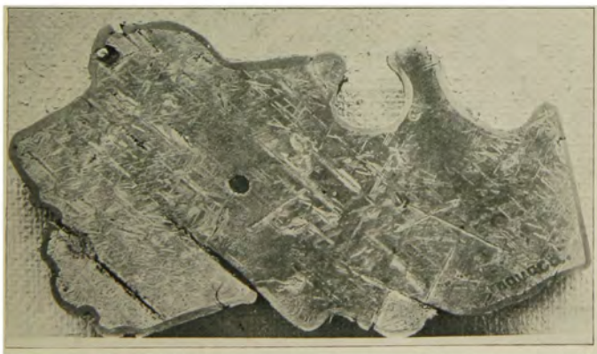
FIG. 2. Section showing Widmanstätten figures. One-half actual size.
