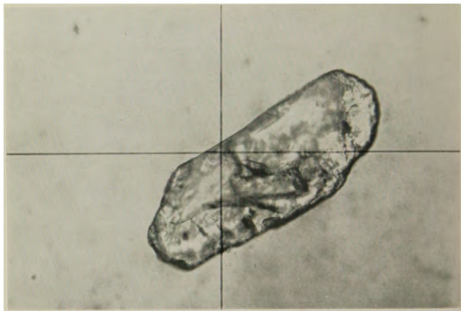
a: Monoclinic Pyroxene (1000 X) from the Albion-Rochester moraine. Note the well-rounded ends and the fresh appearance.
