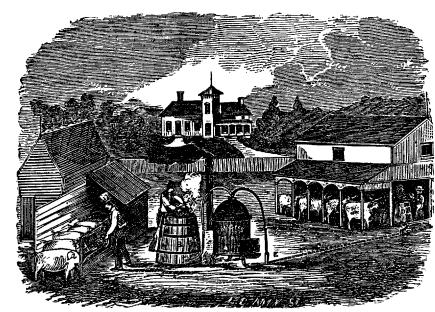
This Engraving represents the Apparatus for Cooking large quantities of Feod for Stock at a time, and at any point desired, through a pipe or log in the ground or otherwise, extending to the barn or any other point, as represented by E, C, thus avoiding all danger from fire. This is the principal use for which it was first projected by the Patentee.
