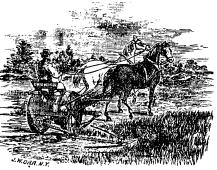
1. The carriage of the machine is mounted on two driving wheels. In connection with each of these is a spur wheel and pinion, making the machine stronger and more durable than any single-geared machine can be.
