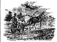
1. The carriage of the machine is mounted on two driving wheels. In connection with each of these is a spur wheel and pinion, making the machine stronger and more durable than any single-geared machine can be.
