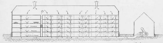
Schematic Drawing Illustrating the Heating and Ventilating of the
