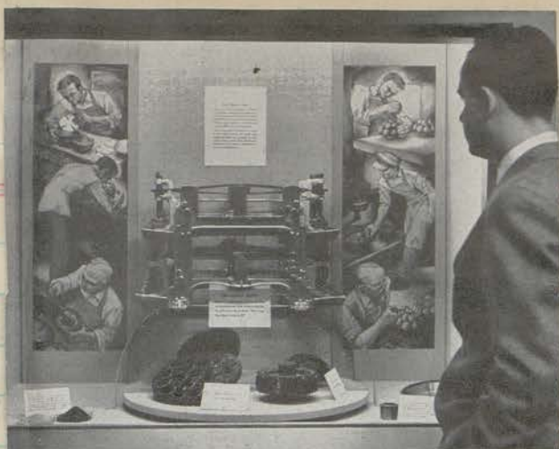
A button-operated model which demonstrates the traditional methods used in grinding and polishing optical surfaces.
