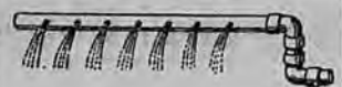
spray installed in the ashpit and connected with the cold water system.
