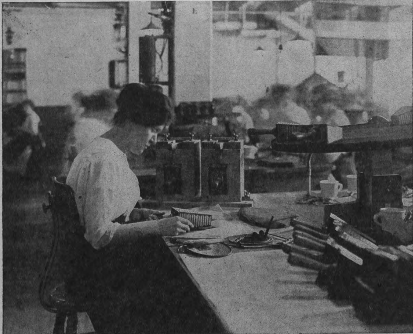
Hundreds of trained hands are employed in the Eastman camera works at Rochester. The operation in the above picture is that of gluing covers on the Kodak bellows.
