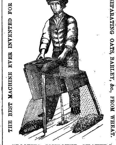
"BOOTH'S COMPOUND SHAKER." For separating Oats, Barley, and other foreign substances from wheat.
