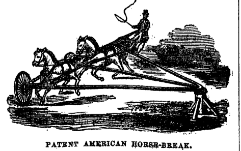
The engraving shows the construction, which is very simple, and it seems to us as well calculated to accomplish the work designed, as the horse can do no injury to himself or the driver,—can neither rear
